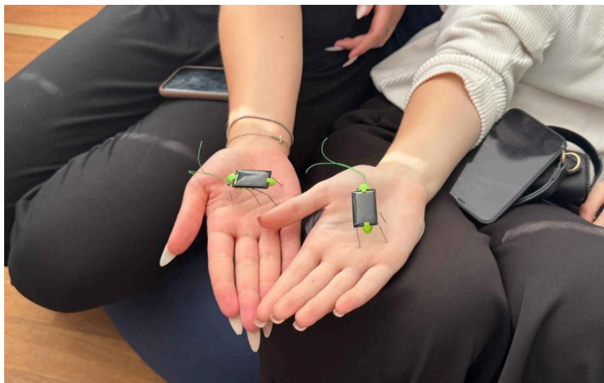
Figure 3 - Instruments for demonstrating solar energy conversion that look like grasshoppers
